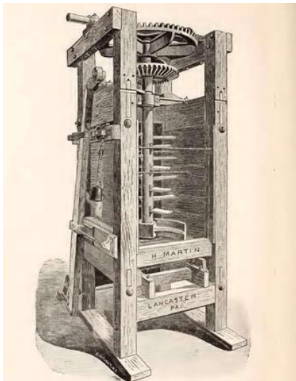
Figure 6: Henry Martin vertical brick machine, 1866 catalog
