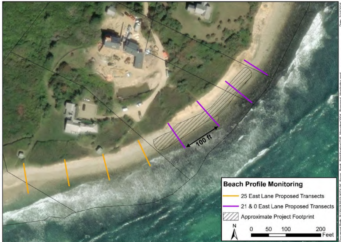
Figure 2. Plan showing location of proposed beach profile monitoring transects at 21 & 0 East Lane.
