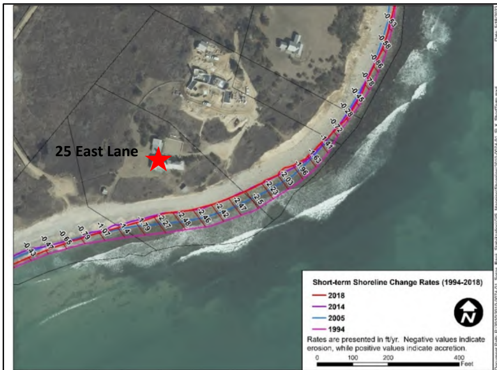
Figure 8. CZM shoreline positions and short-term rates of change from 1994-2018, supplemented with Woods Hole Group data from 2014.
