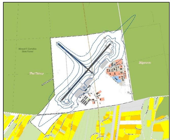
Figure 1. 2028 forecast conditions DNL contours: outermost contour line (dashed) is DNL 60, shown for informational purposes only. FAA's threshold for land use compatibility is DNL 65.
