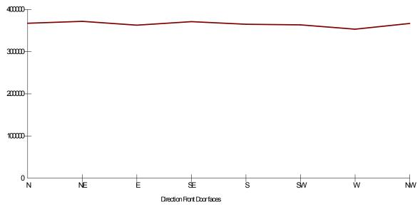
**Current Orientation:** Front Door faces Southeast Highest Cooling Load: Front Door faces Northeast
