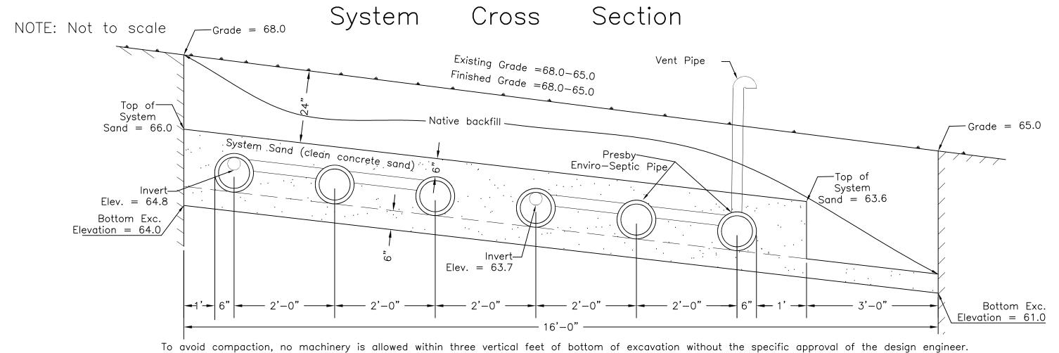
This leaching facility is not designed for H-20 loads and shall not be driven upon
