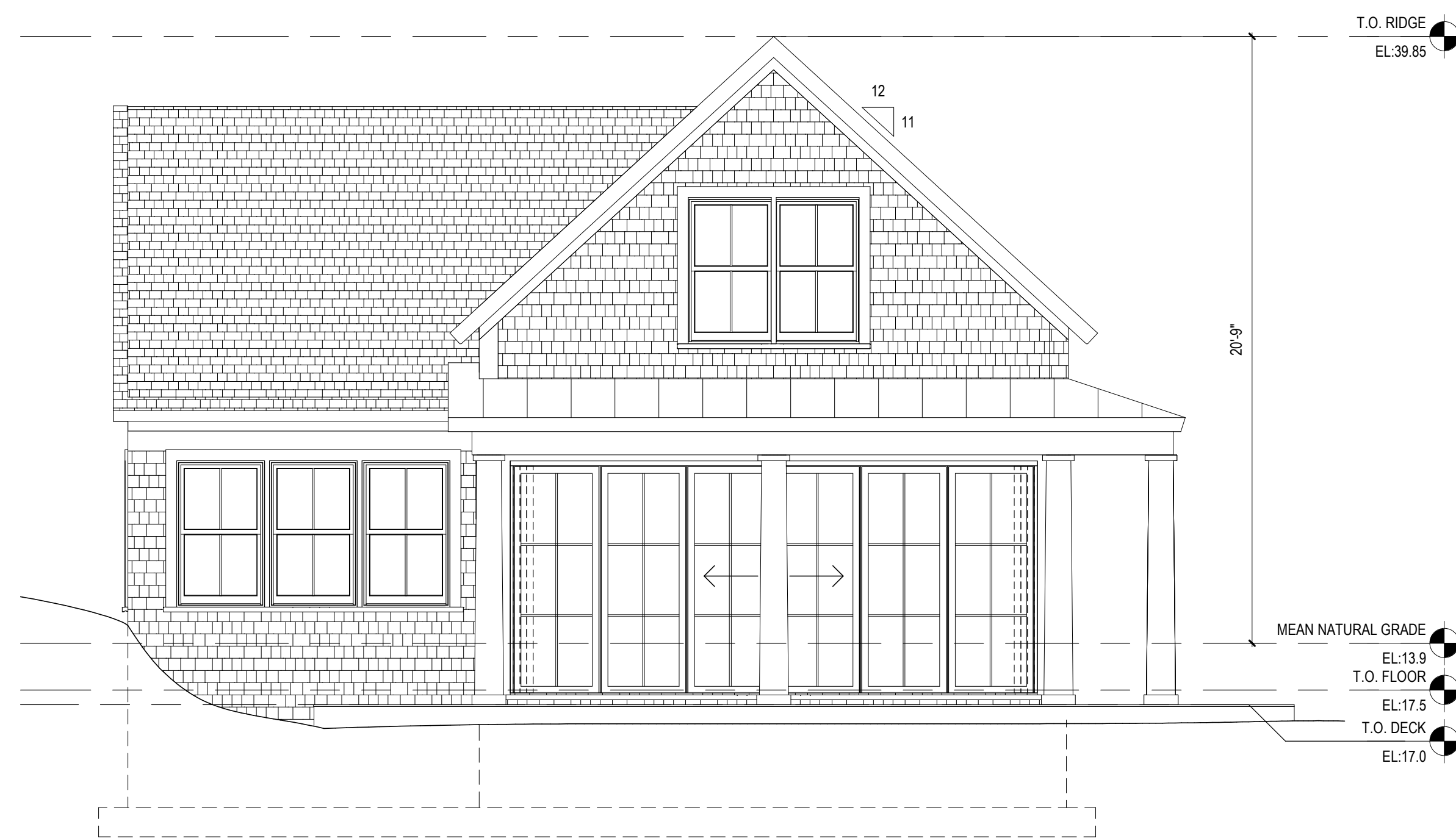
3 POOL HOUSE/GYM EAST ELEVATION SCALE: 1/4" = 1'-0"
