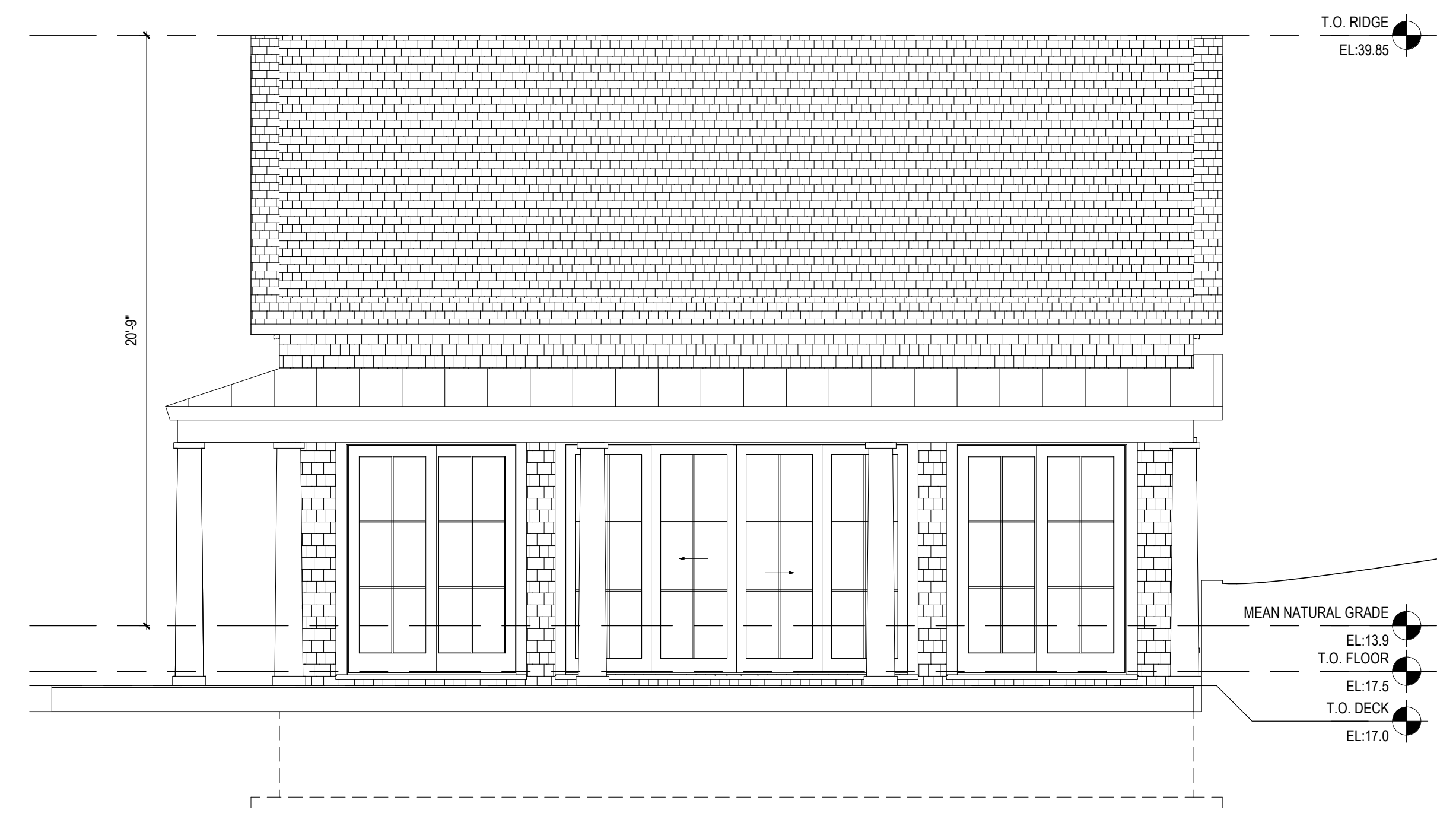
2 POOL HOUSE/GYM SOUTH ELEVATION SCALE: 1/4" = 1'-0"
