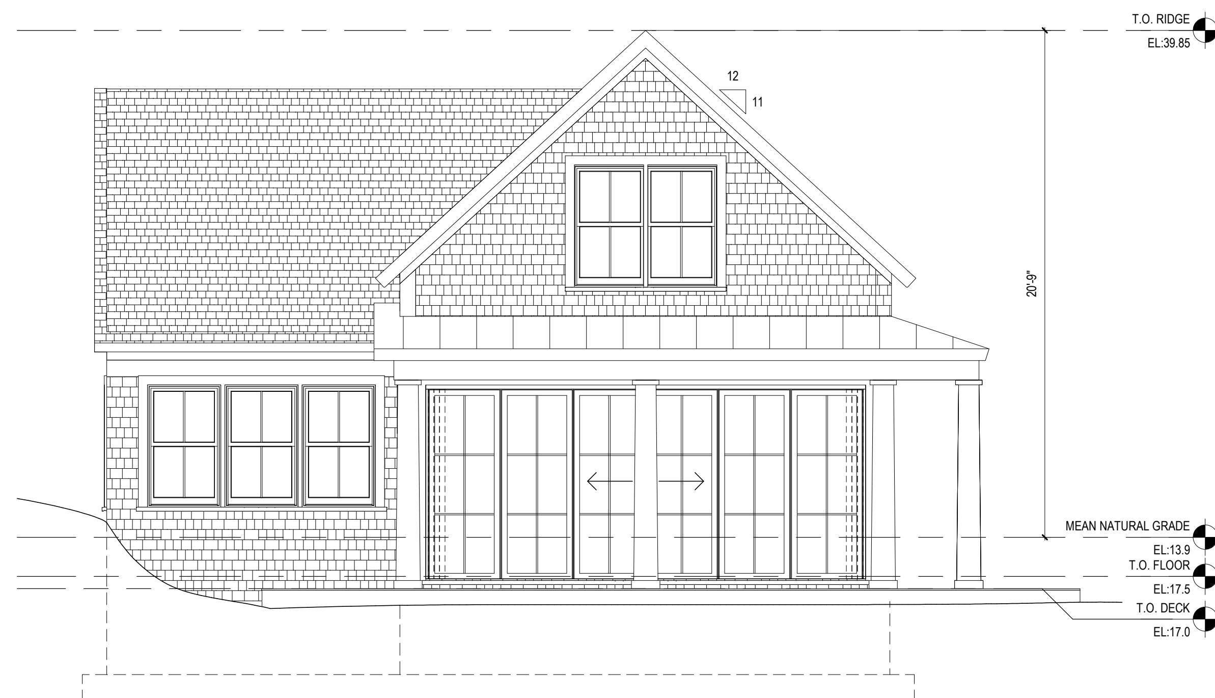
3 POOL HOUSE/GYM EAST ELEVATION SCALE: 1/4" = 1'-0"
