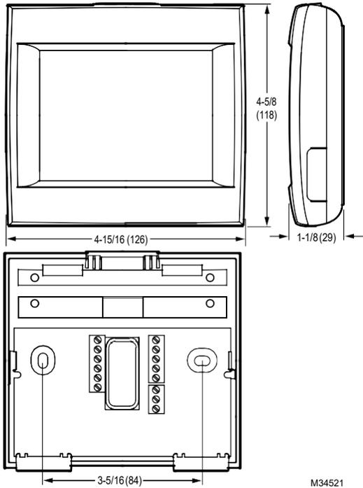
Dimensions of VisionPRO cover plate in in. (mm).
